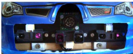
**Fig. 3.** Sensors in the Front of the Unit. From Left to Right, Top to Down, Short Range IR Sensor, Sonar Sensor, Medium Range IR and Short Range IR.
